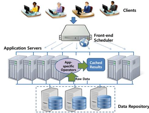
Fig. 1. *Architecture of Distributed Query Processing Framework*
